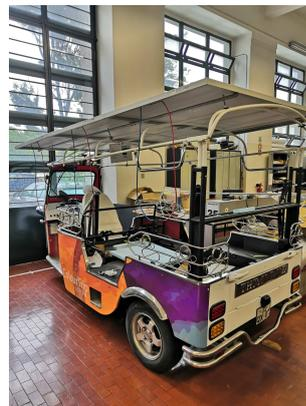
FIG. 4: Setup of the solar photovoltaic panels support.
