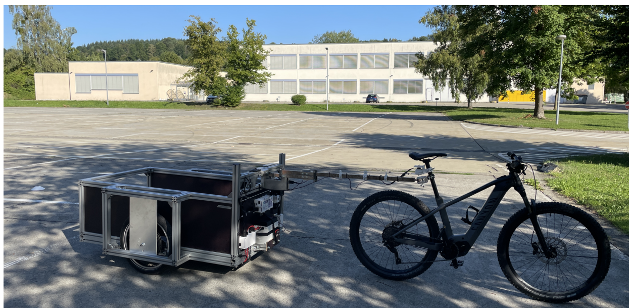
Figure 5. Prototype trailer attached to a bicycle.
