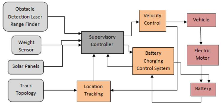
Figure 2. Block diagram of the overall system.
