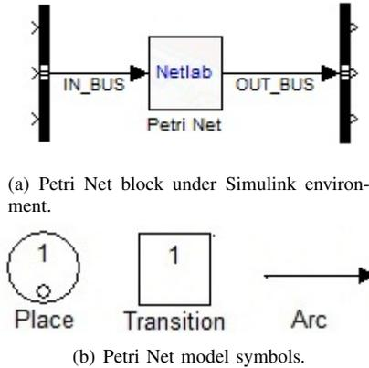
Figure 3. Element symbols from Netlab environment.
