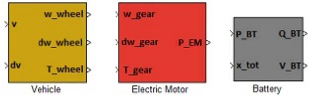
Figure 4. QSS library vehicle, electric motor, and battery blocks.
