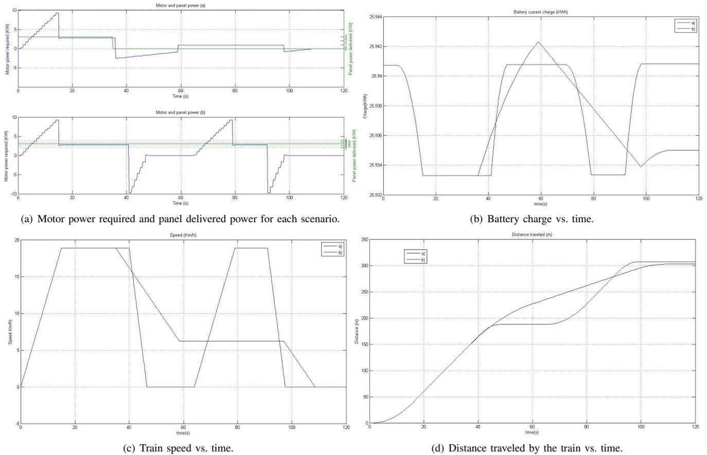
Figure 8. Simulation results for two scenarios: obstacle detection (b) and power cut (a).
