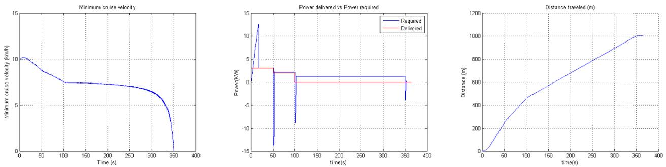
(a) Minimum velocity required to reach the target within schedule.
