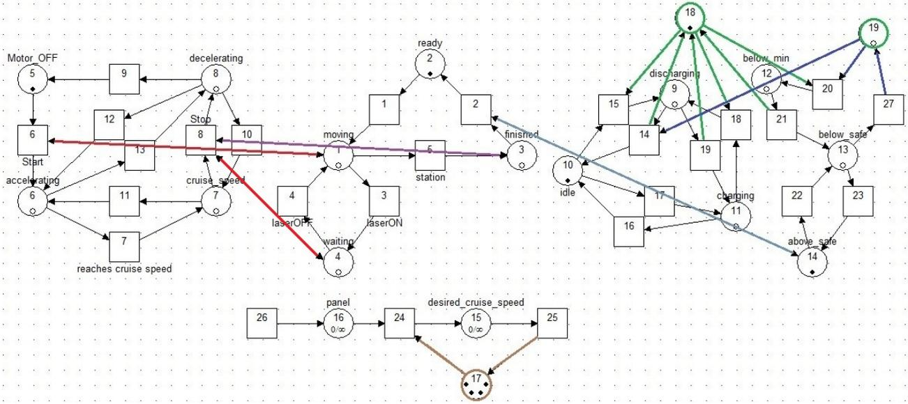
Figure 6. Petri net model of supervised system.
